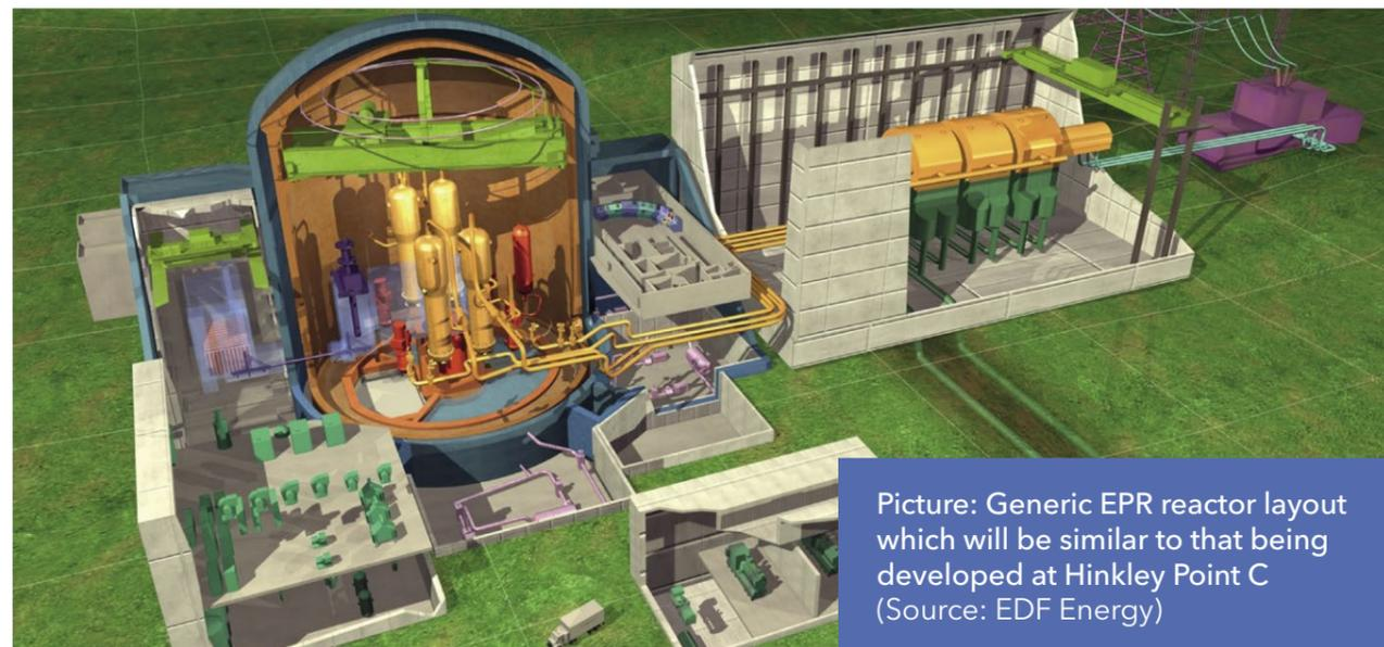
Picture: Generic EPR reactor layout which will be similar to that being developed at Hinkley Point C (Source: EDF Energy)
