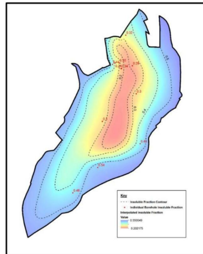
Fig. 8. Mapped insoluble fraction and distribution in the Northwich Halite Member of the Cheshire Basin.
