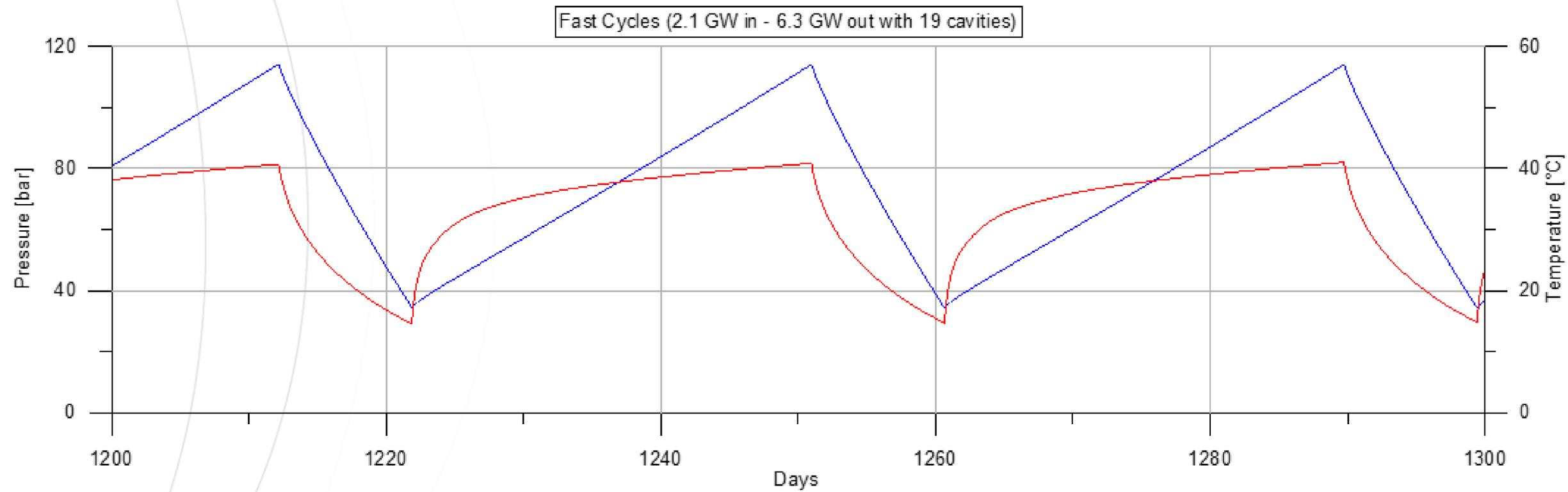
Thermodynamical simulation with hydrogen (Geostock's GUSTS software)
