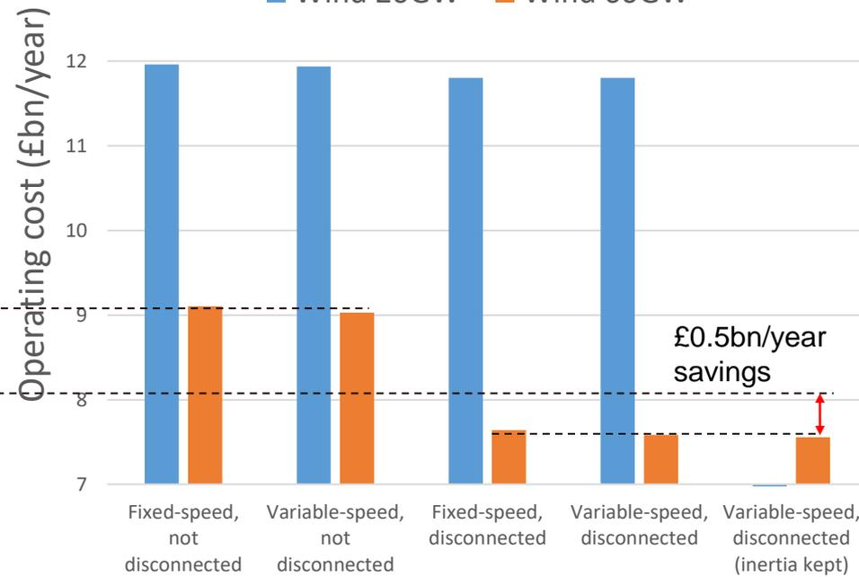
Assuming that ES units in charging mode could **provide fast frequency response** by disconnecting after an outage, and potentially **provide inertia**
