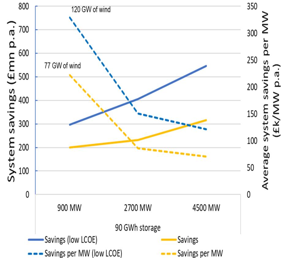
Increased wind (e.g. driven by lower wind LCOE ) will intensify the benefits of MDES especially with long duration capacity
