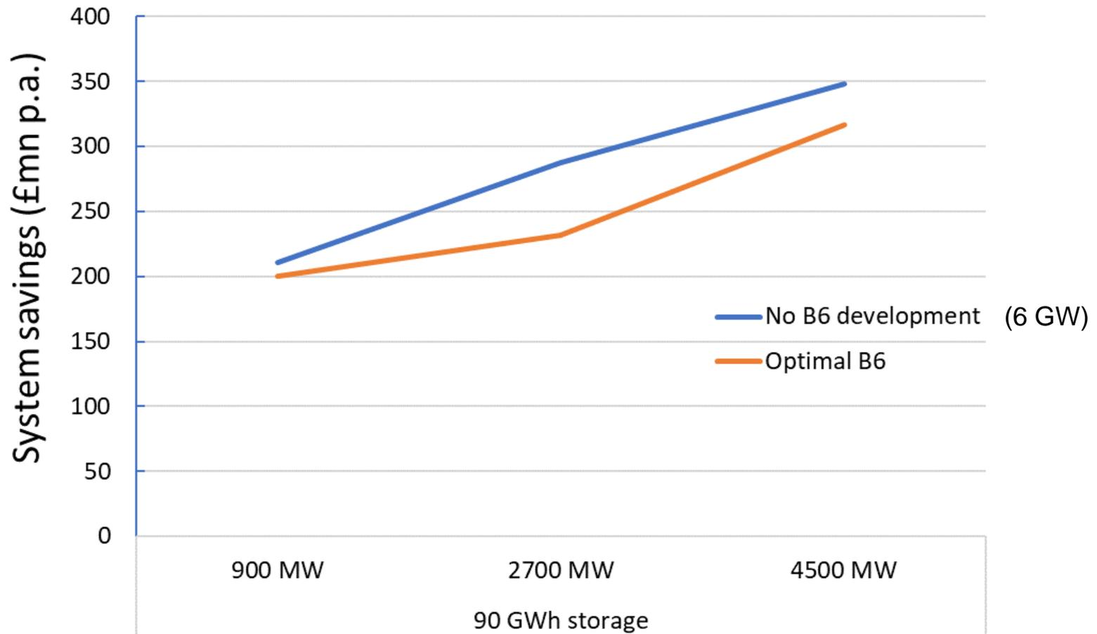
Value of MDES is higher if transmission capacity is suboptimal
